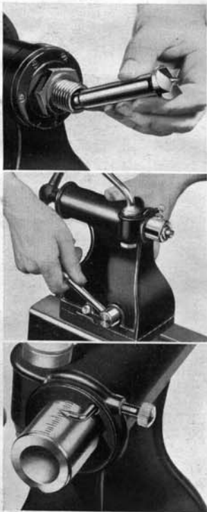
Top, inserting the spur center in the hollow headstock spindle. Center, releasing the tailstock clamp. Bottom, the tailstock spindle is graduated as an aid in taking dimensions.
